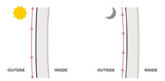
If the hooks on the multipoint lock are not thrown throughtout the day and the centre keep setting is too tight, the top and bottom of the door will be in unsupported tension and will eventually stand proud of the inner face of the profile. This will make the hooks on the lock become stiff, as they cannot draw themselves into the hook keep.
