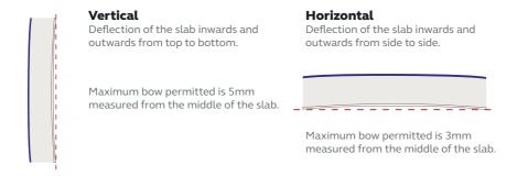
Slackening off the lock keeps will compensate for the movement of the slab within these tolerances. The hooks of the multipoint lock must be in compression with the inner edge of the pocket keep. If this does not happen the door may move to the inside or the property (towards the cold side) and give the impression the door is bowed.
